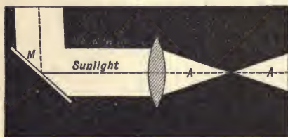
FIG. 236. — Effect of a Convex Lens on Parallel Rays.
